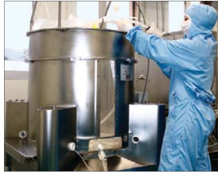
Adolf Kühner's SB200-X is a disposable shaking bioreactor system for cell cultivation. It was developed and tested in cooperation with ExcellGene and UNIL-EPFL.
