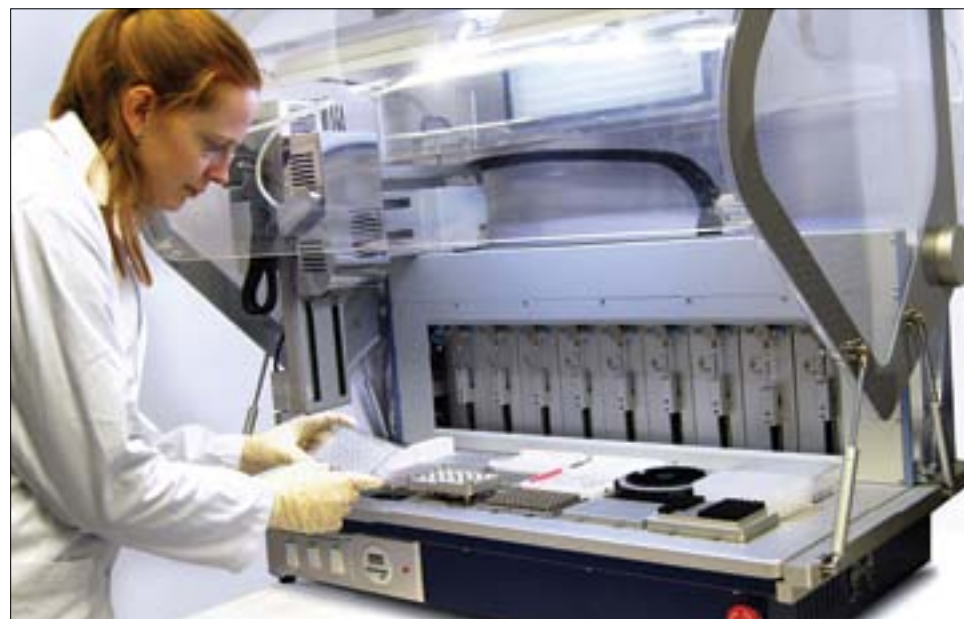
According to Aurora Biomed, its Versa 1100 automated, multichannel, liquid-handling system maximizes accuracy, precision, and throughput while minimizing time and consumable costs. It also offers flexibility in volume range, liquid-handling modules, deck modules, and labware adapters for custom applications used in specific protocols.
