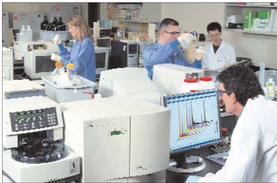
ESA Biosciences' CoulArray system relies upon the electroactive nature of molecules—a molecule's ability to be oxidized or reduced. The technology lends itself to the analysis of xenobiotic molecules and charged or uncharged pharmaceutical compounds.
