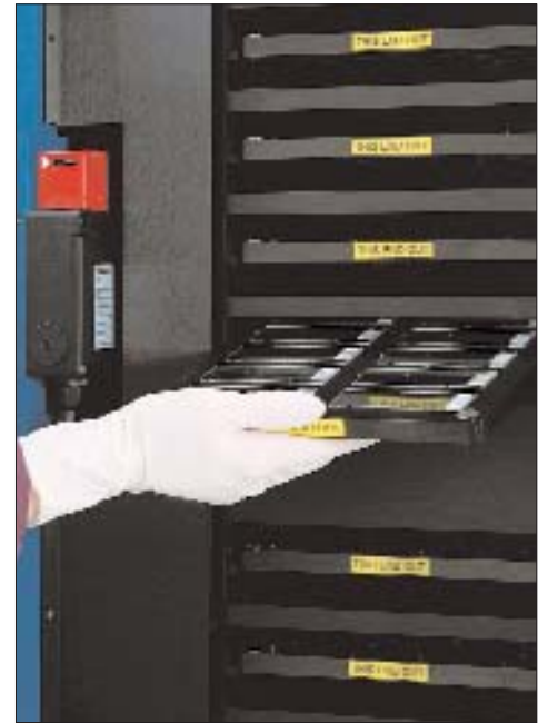
Aushon Biosystems' 2470 Arrayer is a high-throughput microarrayer designed to provide rapid, high-quality printing of a wide variety of materials, including cell lysates, onto most any substrate. Substrate platens such as the microscope slide platens in this photo are housed in the substrate elevator and printed sequentially, allowing for walk-away automation.
